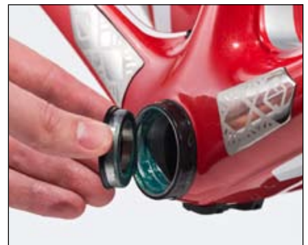
Figure 49. Pressing the bearing into the frame with the shield on the outside
